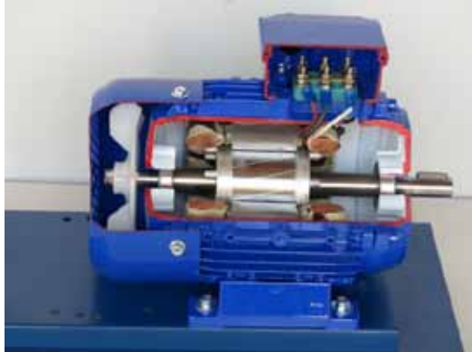
Mod.3040 Three Phase Squirrel Cage Motor
