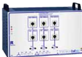
Mod.4020-110R Load resistive for dynamo & alternator; Starter for DC motor.; • Variable 3x 1%÷110%; • 3Ph: variable with 110 steps from 1% to 110% • Power: 10÷1000VA; Triphase / monophasé; (monophasé with 330 steps);
