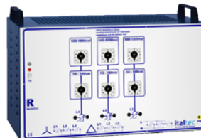
Mod.4020-110R Load resistive for dynamo & alternator; Starter for DC motor.; • Variable 3x 1%÷110%; • 3Ph: variable with 110 steps from 1% to 110% • Power: 10÷1000VA; Triphase / monophasé; (monophasé with 330 steps);
