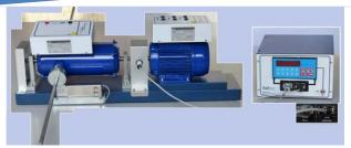
This meter allows to measure the motor torque during the test and to read the torque and the speed values on the digital instrument display. For use with brake generator, electromagnetic brake or brake generator. Torque can be read in kgm or Nm.
