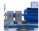
Rotating torque transducer for torque detection
